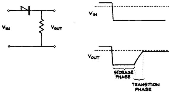
Fig. 1. Single-diode pulse generator.
