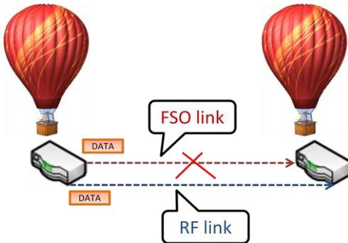
**Figure 4. Misaligned FSO Link; RF as Backup**
