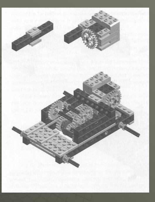
Here you can see the turning motor mounted to the front of the chassis, it connects to the large beveled gear using the small 8 tooth gear at a 90 degree angle.
