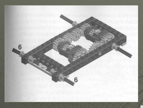
The "Diffbot" uses a double differential design, with 18 gears and two differentials.
