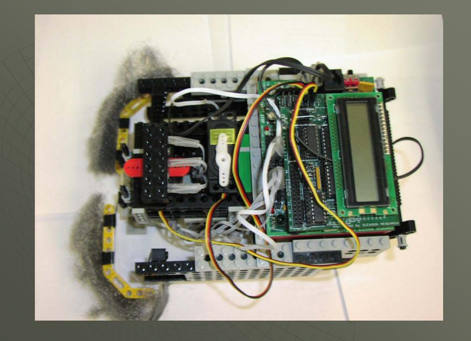
Sensor Placement The touch sensors were mounted in front of the chassis, low to the ground. The light sensors were mounted atop a servo in the front-center of the robot.
