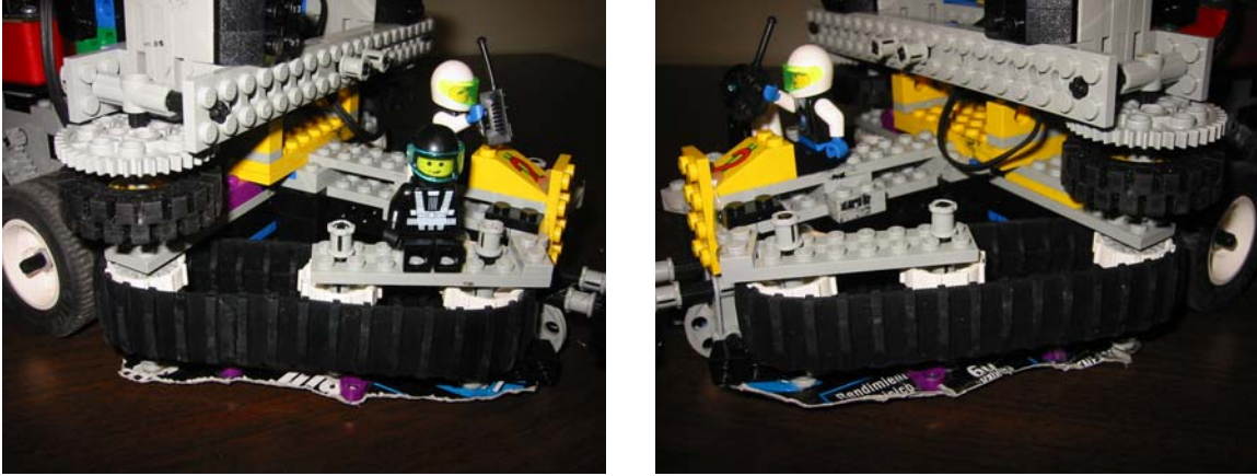
Figure 1.4 – The “Duster” (right and left), motors are mounted vertically connecting to the large 40 tooth gears. Below the gears are the guide wheels.
