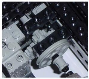
wheel. Together, the gears system and the encoder wheel generate 36 ticks for a single wheel revolution. This resolution breaks down to one tick being approximately  $3/16^{\text{th}}$  of an inch.
