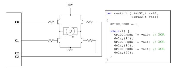
Assume that Port C, pins 0..3 are configured as digital output pins. Also assume that the motor can be modeled as a  $2\Omega$  resistor.
