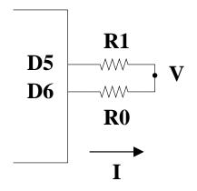
Assume  $R_0 = 50\Omega$ ,  $R_1 = 200\Omega$  and the maximum voltage output by a microprocessor pin is 5V.
