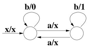
This FSM has the following inputs: x, a, b, and the following outputs:
