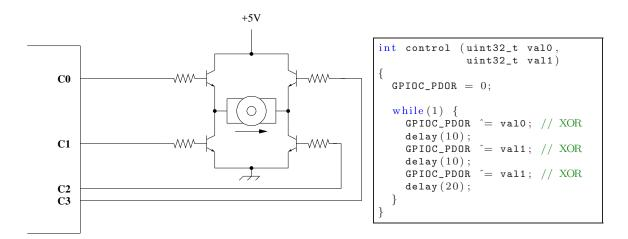
Assume that Port C, pins 0..3 are configured as digital output pins. Also assume that the motor can be modeled as a  $2\Omega$  resistor.
