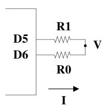
Assume  $R_0 = 50\Omega$ ,  $R_1 = 200\Omega$  and the maximum voltage output by a microprocessor pin is 5V.
