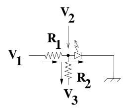
Assume  $R_1=100~\Omega,~R_2=300~\Omega$  and  $V_f=1~V.$
