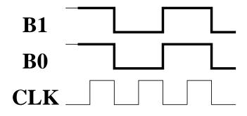
(b) (5 pts) Assume that the initial state is B1 = 0 and B0 = 1, and that A = 1. Fill in the following timing diagram:
