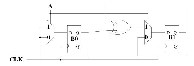
(a) (5 pts) Assume that the initial state is B1 = 1 and B0 = 1, and that A = 0. Fill in the following timing diagram:
