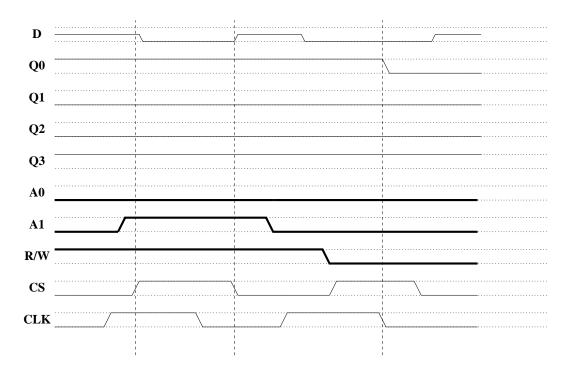
Note: we were pretty liberal about grading the timing diagram. In addition to having the signals be in the correct states (at certain times), we looked for having the signals be set up in time for the read or write operation. Specifically, the address and R/W lines needed to be configured before the chip select line went high.
