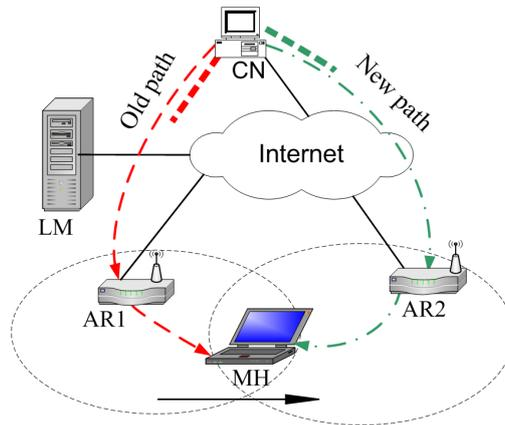
**Figure 2** HMIPv6 architecture (see online version for colours)
