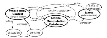
Figure 1: Overview of the system components implemented for the proof of concept presented in this paper, with arrows denoting information flow.
