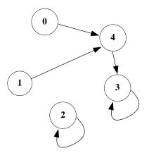
One way to represent the transition function encoded by the arrows in this figure is through a table. For this FSM, the transition function is:
