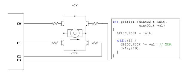
Assume that Port C, pins 0..3 are configured as digital output pins. Also assume that the motor can be modeled as a  $1\Omega$  resistor.
