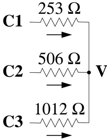
$C1$ ,  $C2$  and  $C3$  are digital output pins from a microcontroller. Assume that  $C_i \in \{0, 1\}$  and are all known.
