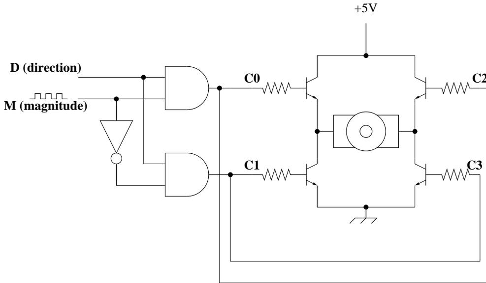
$D$  is a directional input that is intended to specify the direction of motor torque.
