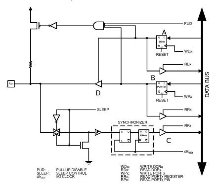
(a) (8 pts) Identify component "C". Explain in brief the function of this type of component (in general, not in this circuit).
