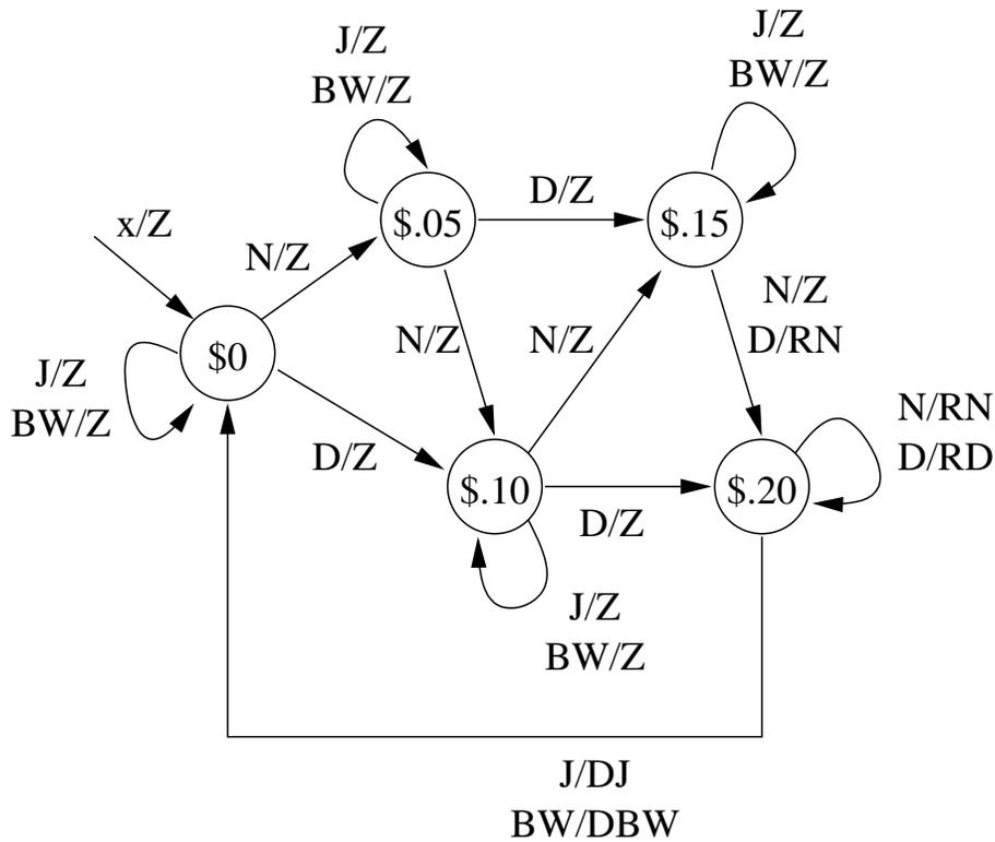
Where the events are: N = Nickel (insertion); D = Dime (insertion); J = Jolt (request); BW = Buzz Water (request).
