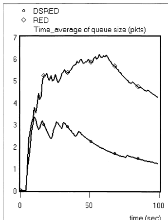
Fig. 11 Time average of queue size for DSRED and RED under Heavy Load for \gamma = 0.91 and Max_{drop} = 0.2 .
