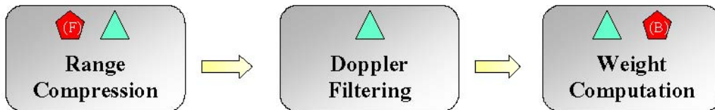
Figure 3. Major computational components of STAP processing flow.
