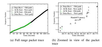
Fig. 7. Packet trace of SIGMA handoff.
