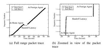
Fig. 5. Packet trace of Mobile IP handoff.
