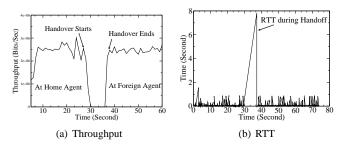
Fig. 4. Throughput and RTT of Mobile IP handoff.
