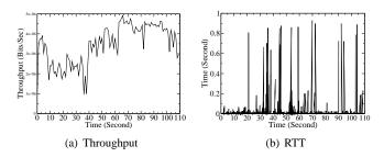
Fig. 6. Throughput and RTT of SIGMA handoff.
