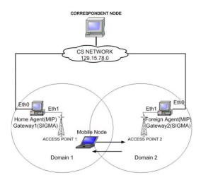
Fig. 3. SIGMA and Mobile IP testbed.
