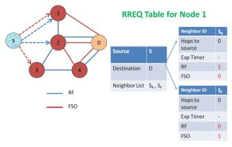
Figure 6. RREQ Table for Node 1 (stage 1)
