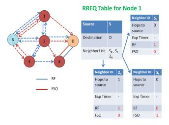
Figure 7. RREQ Table for Node 1 (Stage 2)
