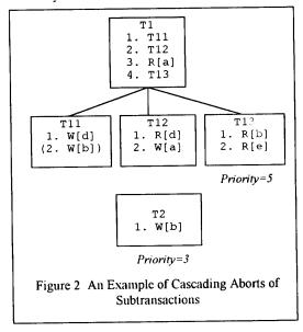
From the above example, aborting subtransactions can cause other subtransactions of the same family to be aborted, and even though some of these subtransactions may have committed. Therefore, an efficient search method needs to navigate through a transaction tree to determine which subtransactions should be aborted when a subtransaction aborts.
